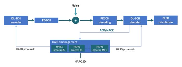
This figure shows that the DL-SCH encoder uses internal buffers to store the transport blocks for each HARQ process and then selects the active HARQ process buffer content for the encoding. The DL-SCH decoder uses a similar buffering mechanism to store and select HARQ processes.
