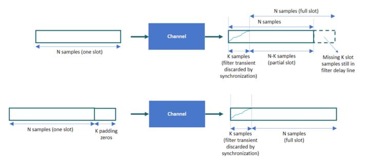
Pad the input signal with enough zeros to ensure that the generated signal is flushed out of the channel filter.
