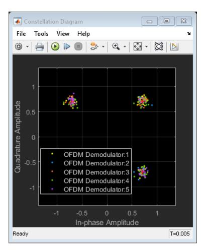
After demodulating the OFDM waveform by using the OFDM Demodulator block, the Constellation Diagram block displays the resulting QAM symbols.
