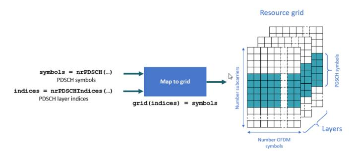
Because this example applies MIMO precoding to the PDSCH symbols before mapping them to the resource grids, the MIMO-precoded PDSCH symbols refer to antennas and not layers. To convert layer indices to antenna indices, use the nrExtractResources function. This figure shows the mapping process of MIMO-precoded symbols to as many resource grids as transmit antennas.
