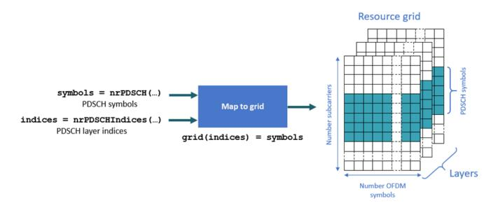
Because this example applies precoding to the PDSCH symbols before mapping to the resource grid, the precoded PDSCH symbols are mapped to antennas and not layers. To convert layer indices to antenna indices, use the nrExtractResources function.
