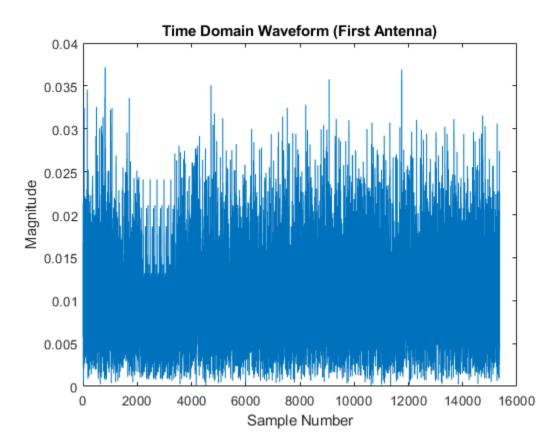
The waveformInfo output contains information about the time-domain waveform, such as the sampling rate.
