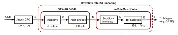
For the downlink, the input bits are interleaved prior to polar encoding. The CRC bits appended at the end of the information bits are thus distributed for the CA-Polar scheme. This interleaving is not specified for the uplink.
