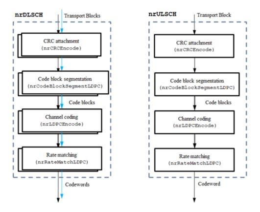
Refer to nrDLSCH and nrULSCH System objects that encapsulate the processing per transport block, with additional support for retransmissions.
