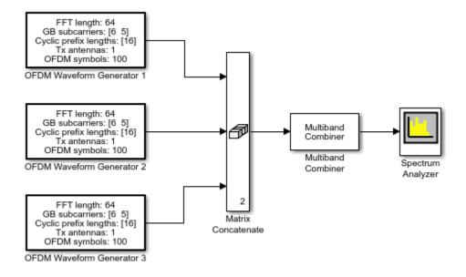
To shift the waveforms in frequency, you might have to increase the sampling rates. The Multiband Combiner block provides the option to oversample the input waveforms before shifting and combining them. This figure shows the parameters of the Multiband Combiner block.
